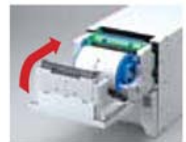
4. Close front door to complete the auto paper loading.
