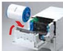
2. Pull out front door and load paper.
